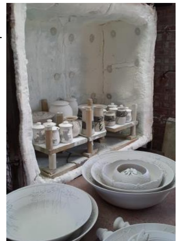
Inside of kiln partly loaded
